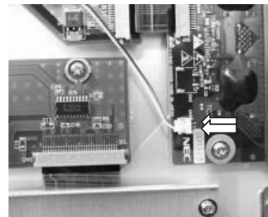
2.4 The conduction between the pins of CN3 on the scan IC [D]
